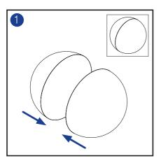
Solder float using WRAS Approved solder/flux.
