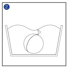
Submerge float and visually inspect. If bubbles are present repeat step 1.
