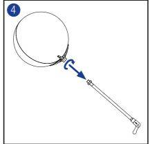
Assemble float to lever by threading together and secure with locknut.
