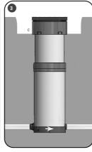
3. Close the lid and backfill with granular material in well compacted 100mm layers to the bottom of the surface box frame (c).
