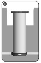
3. Replace the guard tube and cover it to prevent contamination of the chamber and backfill with granular material in well compacted 100mm layers. This needs to be to a level that will allow the fitment of the frame and cover.
