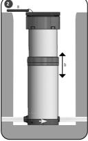
1. The service should be flushed fully to avoid any debris entering the system before connecting the service pipes. Place the complete unit in position on firm even ground and connect the inlet and outlet pipe work (see below). Avoid excess stress being placed on the connections. If necessary use additional fittings to align the pipes. The direction of the flow is indicated by an arrow on the base.
