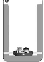
The service should be flushed fully to avoid any debris entering the system before connecting the service pipes. Remove the guard tube from the manifold section and sit the manifold in position on firm ground and connect the inlet and outlet pipework. Avoid excess stress being placed on the connections. If necessary use additional fittings to align the pipes. The direction of flow is indicated by an arrow on the base. Please see EBCO fitting instructions overleaf.
