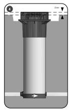
4. Remove the temporary tube cover and ensure any frost protection is fitted inside the tube. Fit the surface box frame and cover raised about 25mm above final surface level. Reinstate backfill material to level of base of surface box/lid assembly. Ensure that the surface box or top hat flange is supported by well compacted backfill material before completing reinstatement to final level.
