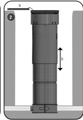
2. Open the surface box lid (a) to allow the telescopic chamber (b) to extend and adjust the box height to the approximate height of the final reinstatement level.
