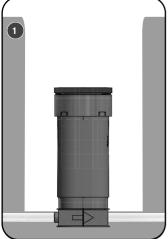
1. The service should be flushed fully to avoid any debris entering the system before connecting the service pipes.
