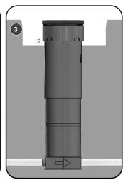
3. Close the lid and backfill with granular material in suitably compacted 100mm layers to the bottom of the surface box frame (c).
