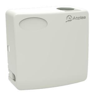
The Atplas Water Point provides a visually elegant, safe environment to house water meters which are installed inside a property. The Water Point consists of a stopcock and a concentric meter port with a built in non-return valve and drain-off point, which can be accessed by removing the front cover of the box. The meter can be read through the lens on the top of the box. The box is large enough to also contain AMR equipment.
