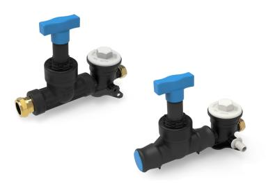
Talbot Internal Meter Carrier Manifolds make it easy to fit concentric water meters internally in a property. Different kits are available to suit various pipework for all applications. The standard kit comes with a Talbot Stopcock (BS5433) on one side and on the other side a Talbot Internal Meter carrier including drain off point BS2464.
