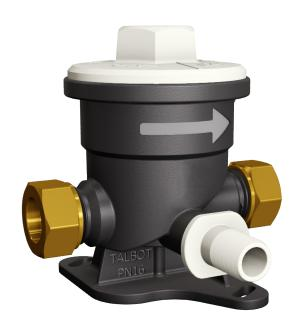
For quick and easy fitting of a concentric water meter inside a property. The carrier comes complete with a non-return valve and drain-off point, for simple and compact fitting and exchange of the meter. The range features different connection sizes for PE and/or copper pipe to fit every installation situation.
