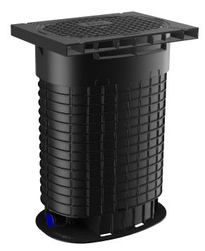
The Matrix Inline range of below ground meter boxes are products that are buried, usually in pavements and walk ways. The Inline range is for use with industry standard inline water meters to a length of 110mm and incorporates quick release meter mountings and a removable stop valve.
