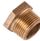
HexBush. Ext. threads: BS21, (BS EN 10226) Int. threads: BS EN ISO 228, (BS2779)
